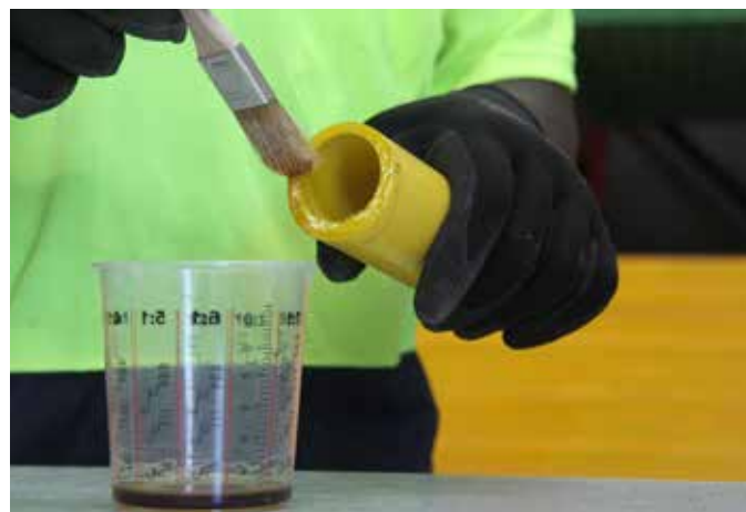
Sealer applied on edges
