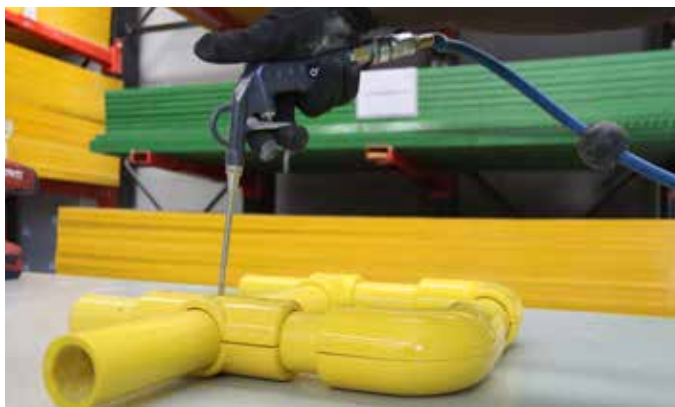
Area is then cleaned with air gun
