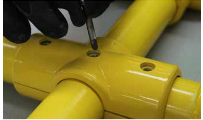
Screws are installed with anti-seize
