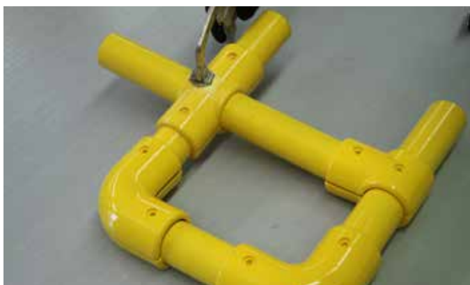
Area to be assembled is first clamped
