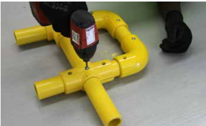
Screws are installed with anti-seize
