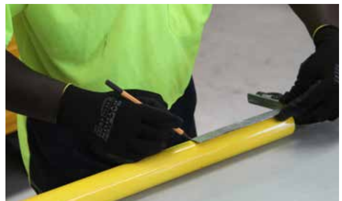
Checking measurement of post throughout
