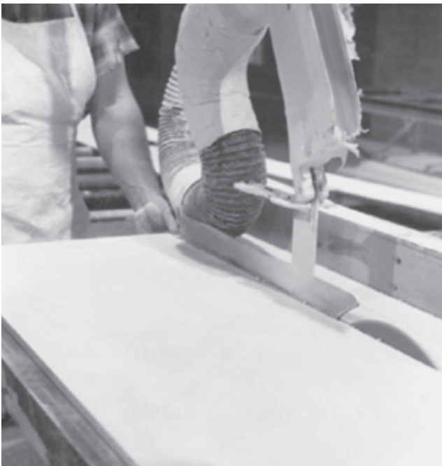
Straight line sawing (vacuum hood raised).
