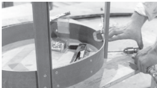
Riveting is a very effective joining method in many applications
